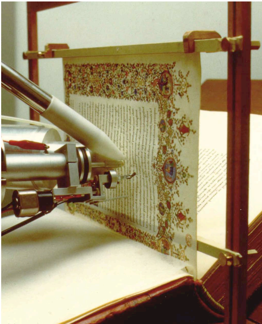
External-beam PIXE analysis of the frontispiece of Pl.16,22, from Biblioteca Laurenziana in Florence
